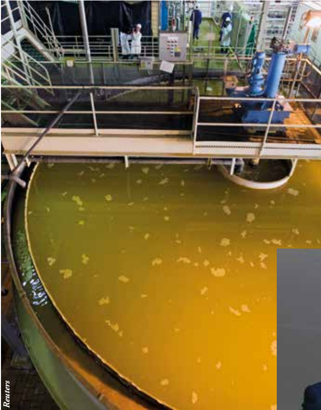
Above: Kazakhstan has abundant resources of uranium. Above is a tank filled with uranium solution at the Inkai uranium mine near the Taikonur settlement in the south of the country.
